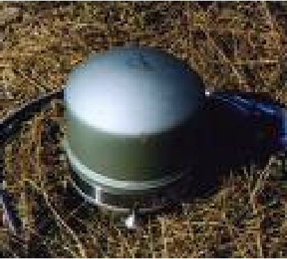
Seismometer to sense earthquakes
